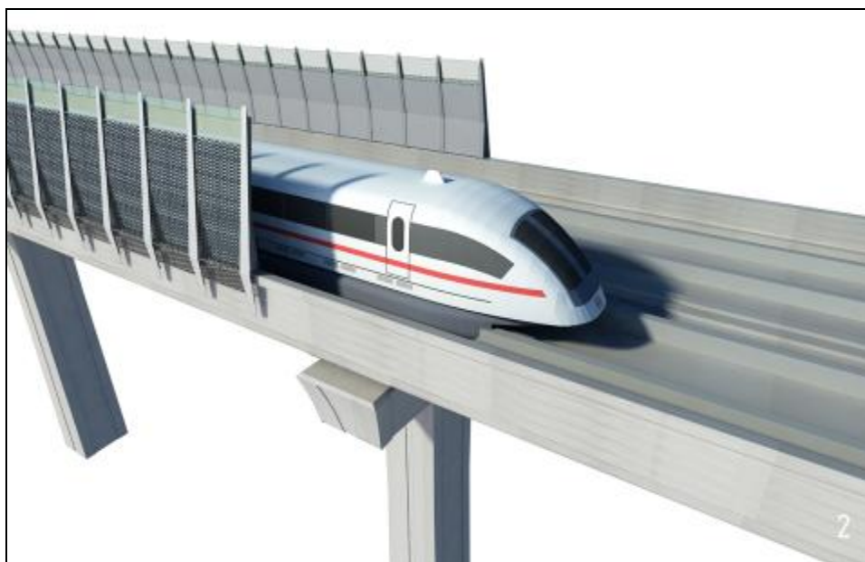
Plate ES-5b Full height noise barrier with architectural aesthetic screen
